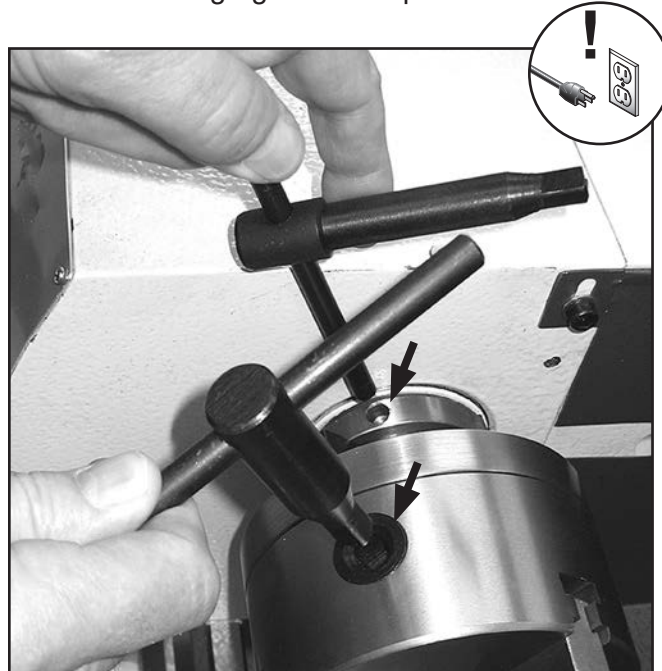
Figure 22. Location to insert chuck keys when installing chuck.
