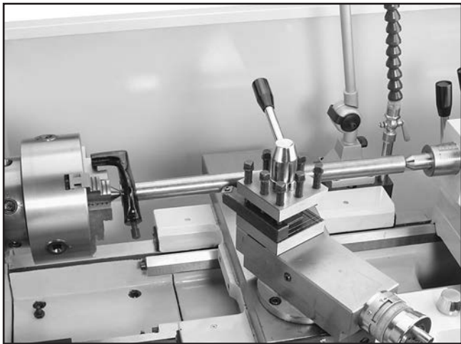
Figure 45. Example photo of a workpiece mounted between the centers.
